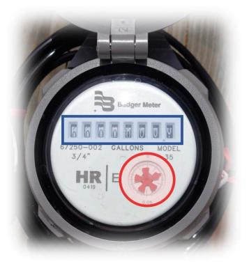
Typical meter display: Low-flow indicator circled in red and register highlighted in blue
